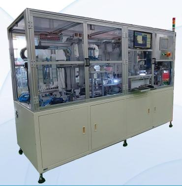
Function introduction : Single test strips, aluminum foil coil continuous automatic feeding / aluminum foil barcode printing / hot pressing / OKNG detection / cutting / sorting collection
